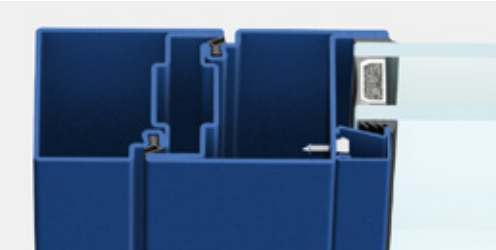
lateral section | frame section 131mm
