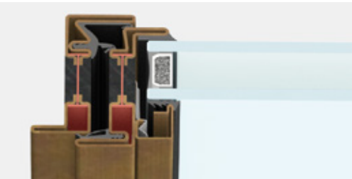
lateral section | frame section 47 mm
