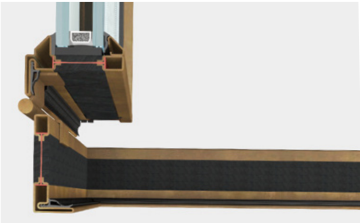
lower section | frame section 47 mm
