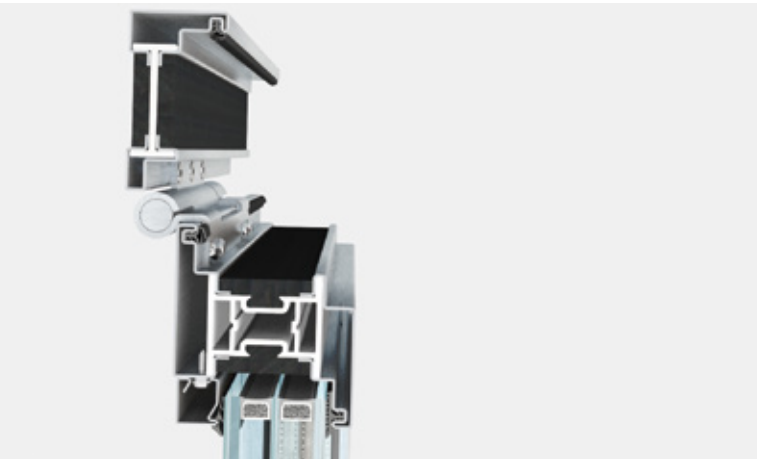
EBE 85 door is an integrated system with accessories, seals and thermal break profiles 85 mm deep allowing for a wide range of windows, rectangular, shaped or curved. They can be equipped with triple glazing up to 60 mm thick.
