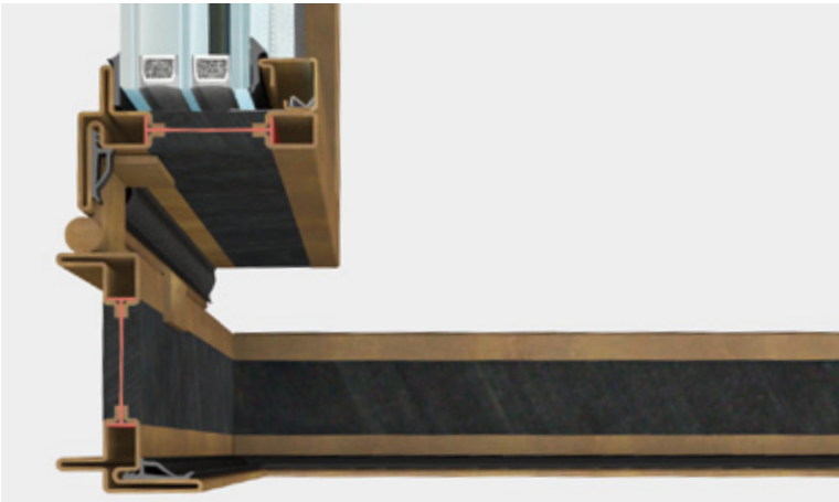
lower section | frame section 47 mm
