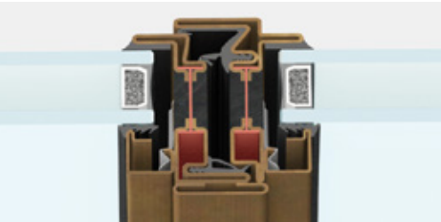
central section | frame section 62 mm
