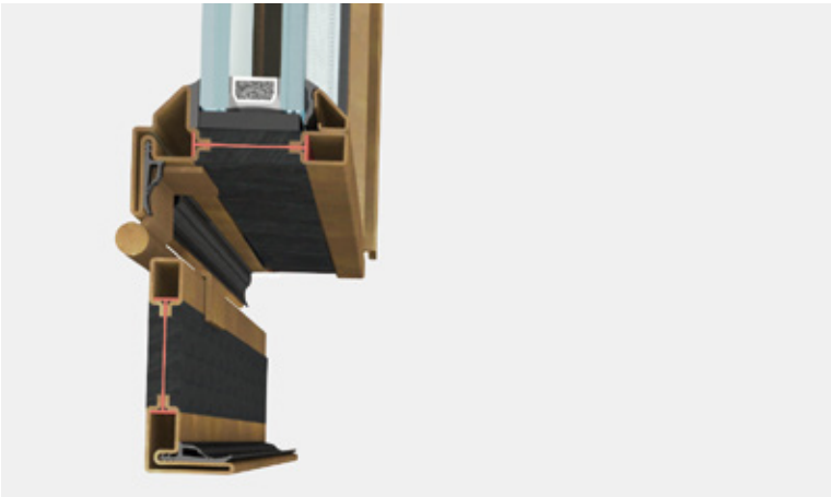
lateral section | frame section 47 mm
