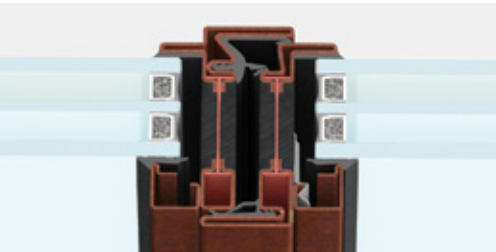
side section | 62 mm visible section
