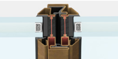
central section | frame section 62 mm
