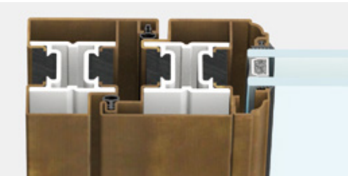
lateral section | frame section 132 mm
