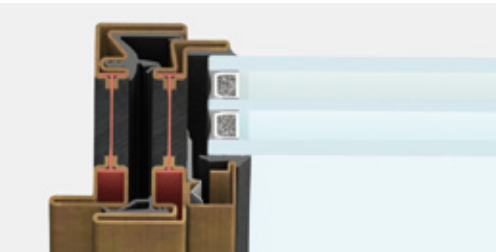
lateral section | frame section 47 mm
