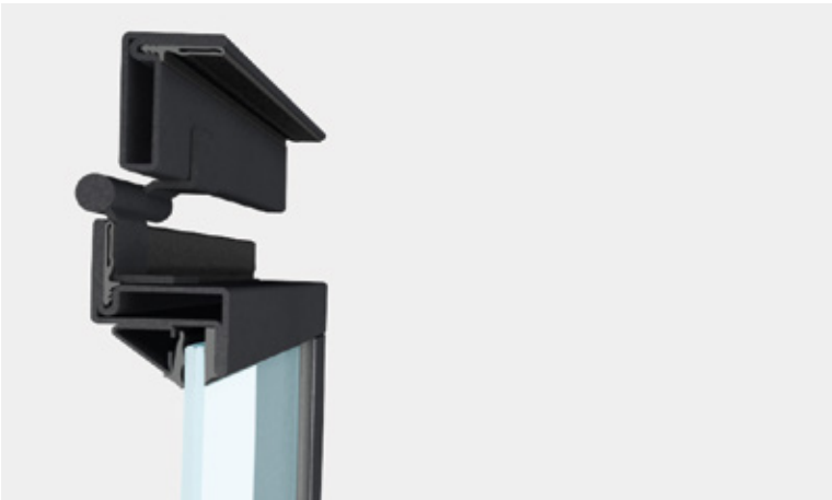
OS2 40 is an integrated system with accessories, seals and profiles 42 mm deep allowing for a wide range of windows, rectangular, shaped or curved. They can be equipped with glazing up to 27 mm thick.
