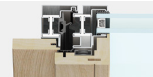
lateral section | frame section 85mm
